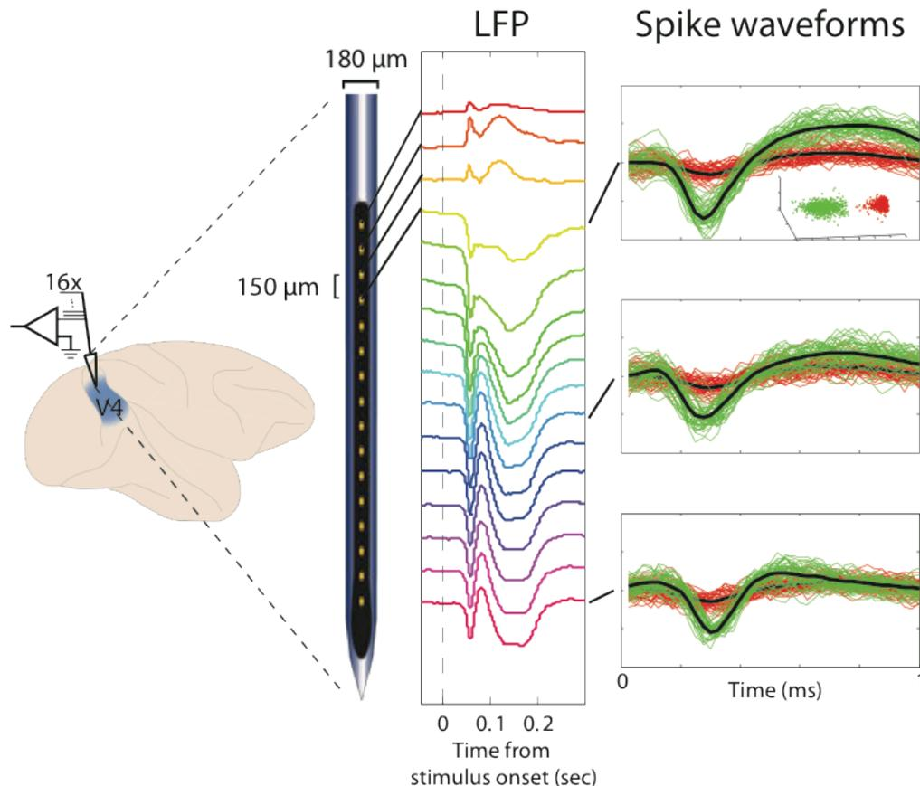
**Figure 4-1. Recording setup, electrode array, and sample data.** Recordings were made from area V4, left panel. Electrodes were 16-channel linear arrays with 150 $\mu\text{m}$  contact spacing. These electrodes were capable of recording LFPs, center, from each channel as well as spikes from isolated single neurons on some channels, right.
