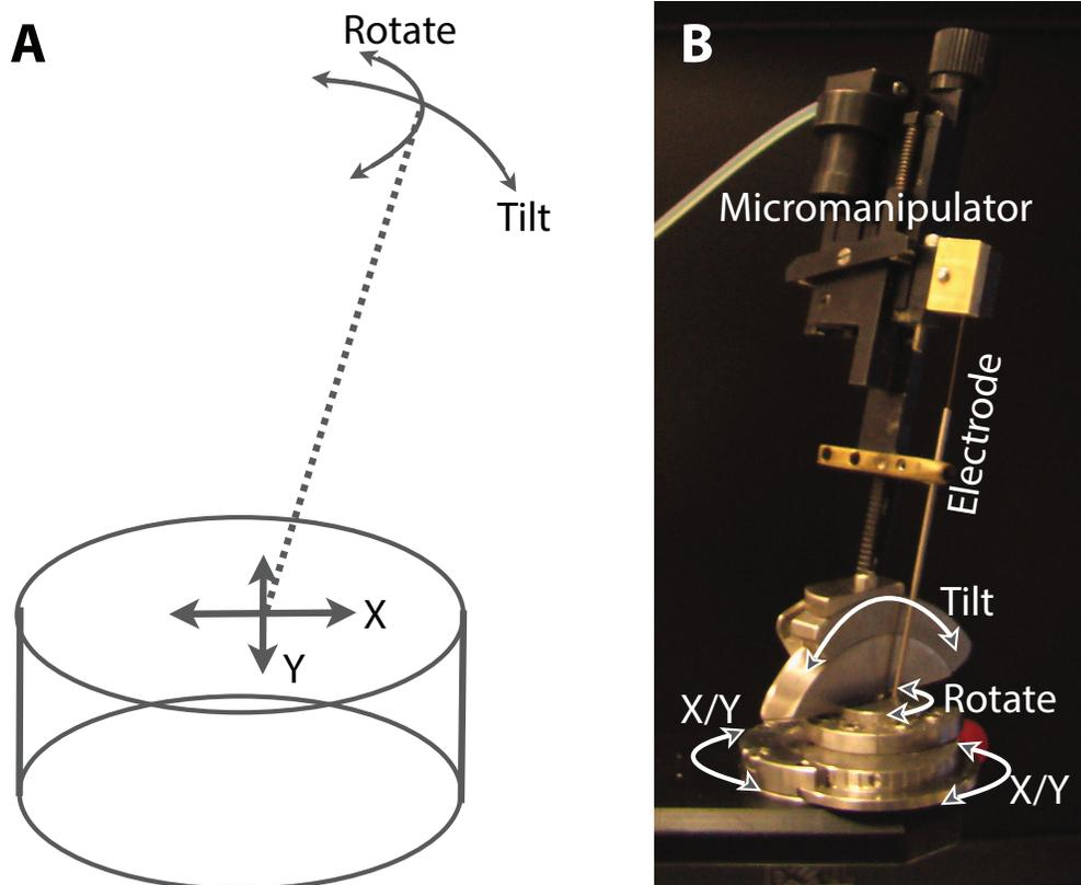
Figure 4-2. “Well angler”: a device to tilt and position an electrode at an arbitrary vector. A, Schematic of recording chamber (cylinder), electrode path (dotted line), and degrees of freedom. B, Photograph of well angler with mechanisms for adjusting degrees of freedom labeled. The Narishige micromanipulator controls
